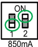
The white squares on the dip switch diagram represent the handle of the dip switch. In the adjacent configuration for 850mA, the white squares have been circled in green to highlight the handle of each switch. To set the driver to 850mA, the handle of switch one should be moved down towards the number 1 and the handle of switch two should be moved up towards ON.
